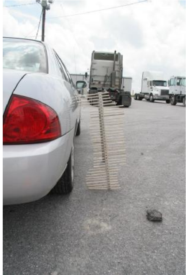
Fig. 12 Matching the profile gauge to the rear fender of an exemplar automobile
