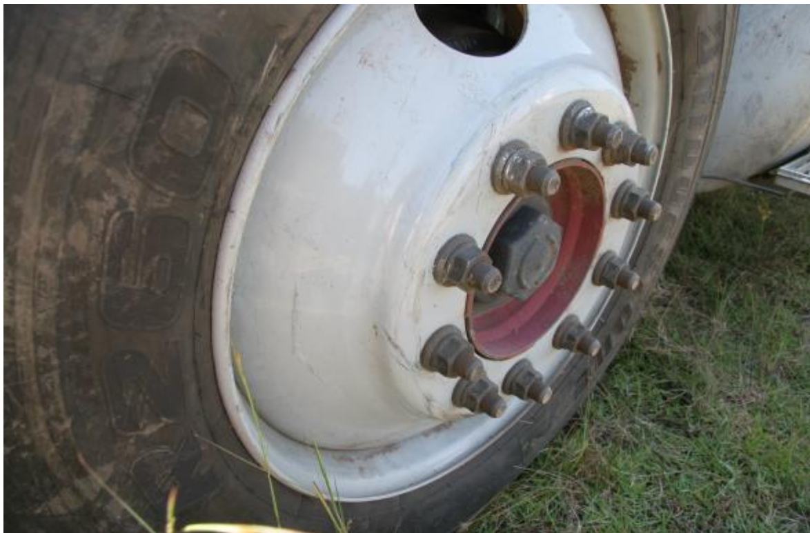
Fig. 5 Left front wheel of the truck; note the protruding lugs
