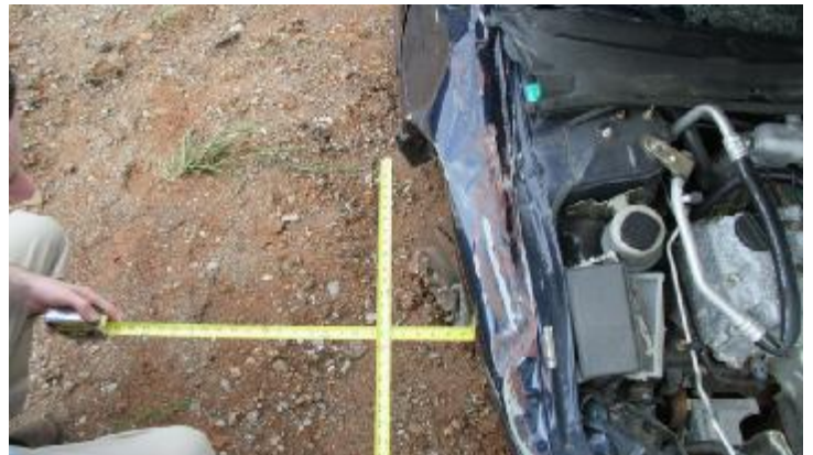
Fig. 2. Measuring the damage pattern on the automobile
