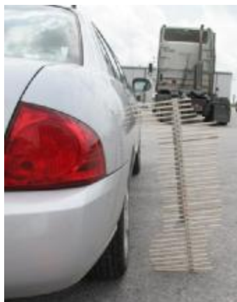
Fig. 4. Matching the profile gauge and a truck against an undamaged exemplar automobile
