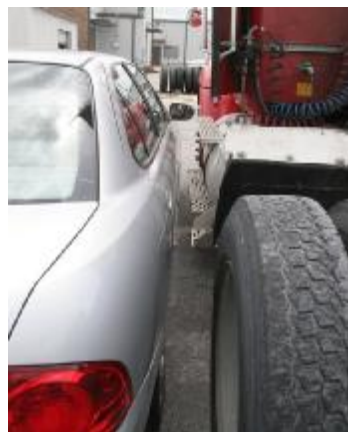
Fig. 4. Matching the profile gauge and a truck against an undamaged exemplar automobile
