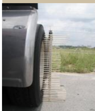
Fig. 3. Using a "homemade" profile gauge to match the truck tire
