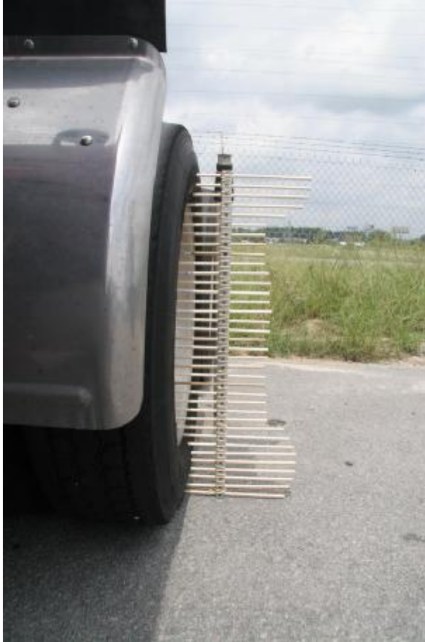
Fig. 11 Matching a "homemade" profile gauge to a truck tire
