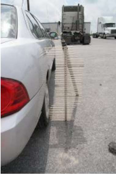
Fig. 13 Using the profile gauge to show the contact pattern if contact had occurred before the truck began the overturn
