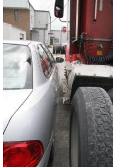
Fig. 14 Exemplar vehicles in a "sideswipe" position
