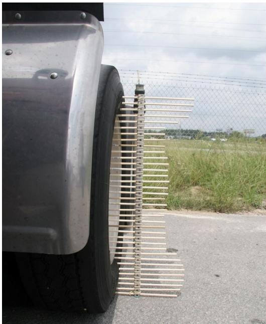
Using a "Homemade" Profile Gauge to Match the Truck Tire
