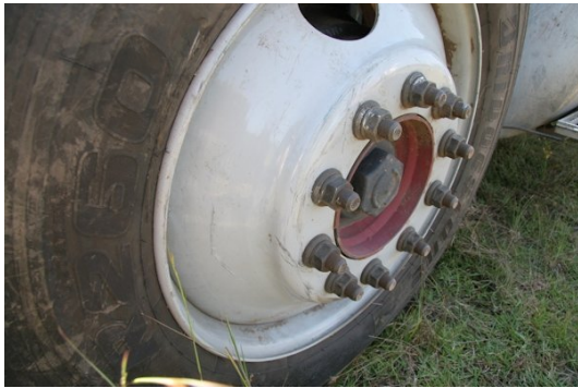
Left Front Wheel - Truck Lug Pattern was Found on Car Passenger Front Fender
