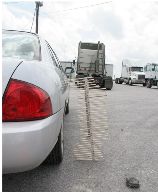
Matching the Profile Gauge To the Fender - Confirming Overturn not Sideswipe
