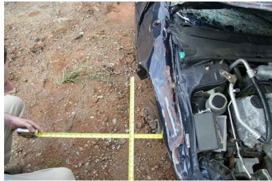
Measuring the Lug Damage Pattern - 20° from parallel
