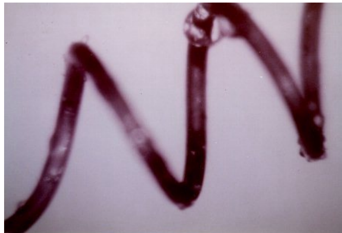
Microscopic view of glass melted onto a filament
