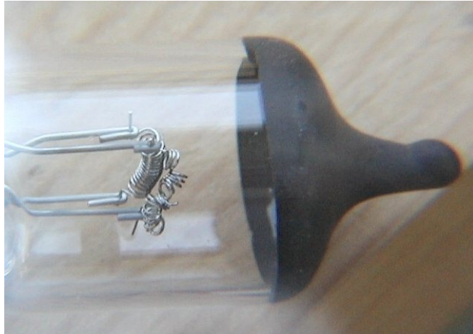
Hot Filament Deformed by Inertial Forces Generated During Impact Notice the Adjacent Undeformed Filament
