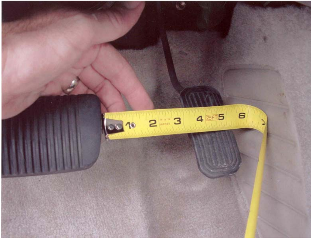
Fig. 8 If the driver momentarily confuses the pedal position, the accelerator is depressed and not the brake. Unfamiliarity is a major cause. This was a rental vehicle.
